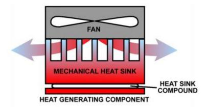
When the gap is not filled properly, the surrounding air can cause a reduction in heat dissipation, leading to device failure. This is because air is a poor thermal conductor. Filling the air gap with the compound improves thermal responsiveness, although heat sink compound does not have the conductivity of metals like copper and silver.
