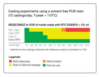
The lower PU-signal of molds **produced with Cata SPU** agrees with casting experiments demonstrating **longer resistance of SPU molds.**
