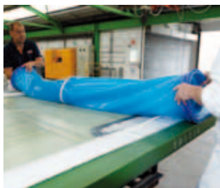
3.1 Removal of bag after curing (2 hours)
