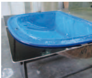
1.4 Spraying the final layer
