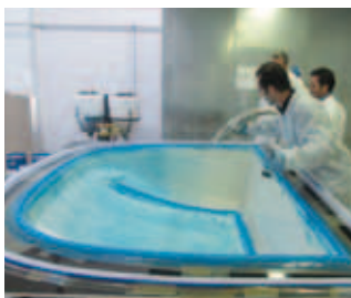
1.2 Spraying of ELASTOSIL® C 1200
