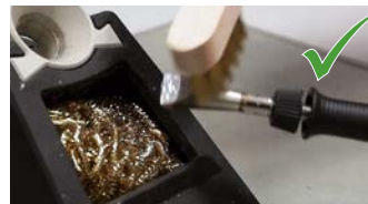
Alternative method: Clean by brass brush (3ZT00051)
