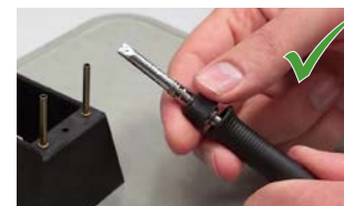
Switch off station, unscrew tip
