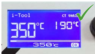
340 – 360 °C for lead-free solder (644 – 680 °F)
