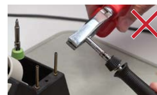
Don't use inappropriate pliers!
