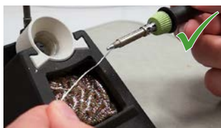
Add new solder after cleaning
