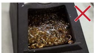
Dirty dry cleaner (flux and oxides)
