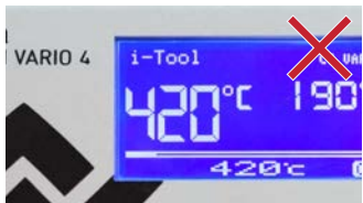
Set reasonable tip temperature!
