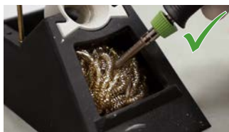
Just stick soldering tip into dry cleaner and turn
