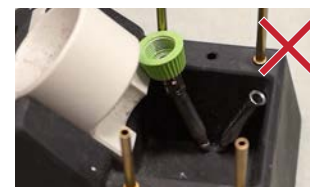
Don't store tips in the stand with opening upwards – dirt may fall in!
