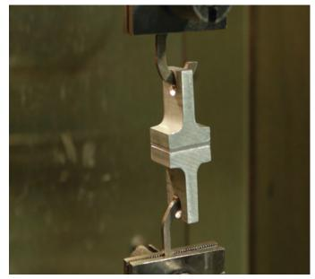
Dynamic normal tensile test: Quantifies the internal cohesive strength of 3M VHB Tape. Unlike mechanical fasteners, the viscoelastic foam core of 3M VHB Tape absorbs the tensile stress, spreading the stress throughout the entire bond.
