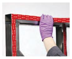
**STEP 2:** When surfaces are dry, apply 3M VHB Tape to the surface.
