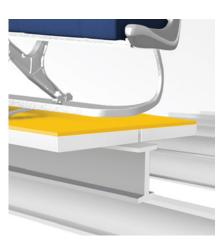
Dual liner tape covers large areas of flooring to prevent fluids from reaching floorboards.
