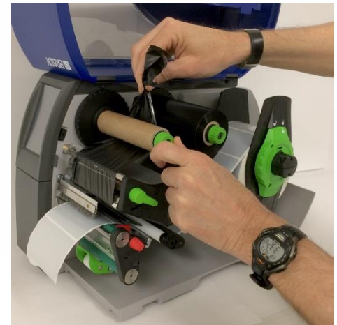
i7100 has extra axle adjustments and you must check ribbon ink first
