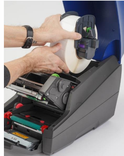
i5100 rolls slide right in...ink always faces the right way
