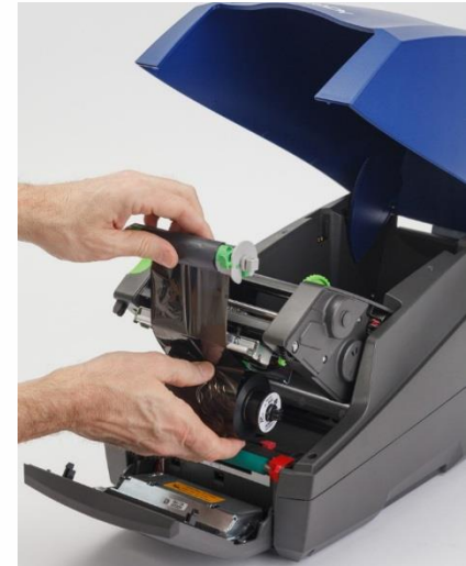
i5100 rolls slide right in...ink always faces the right way
